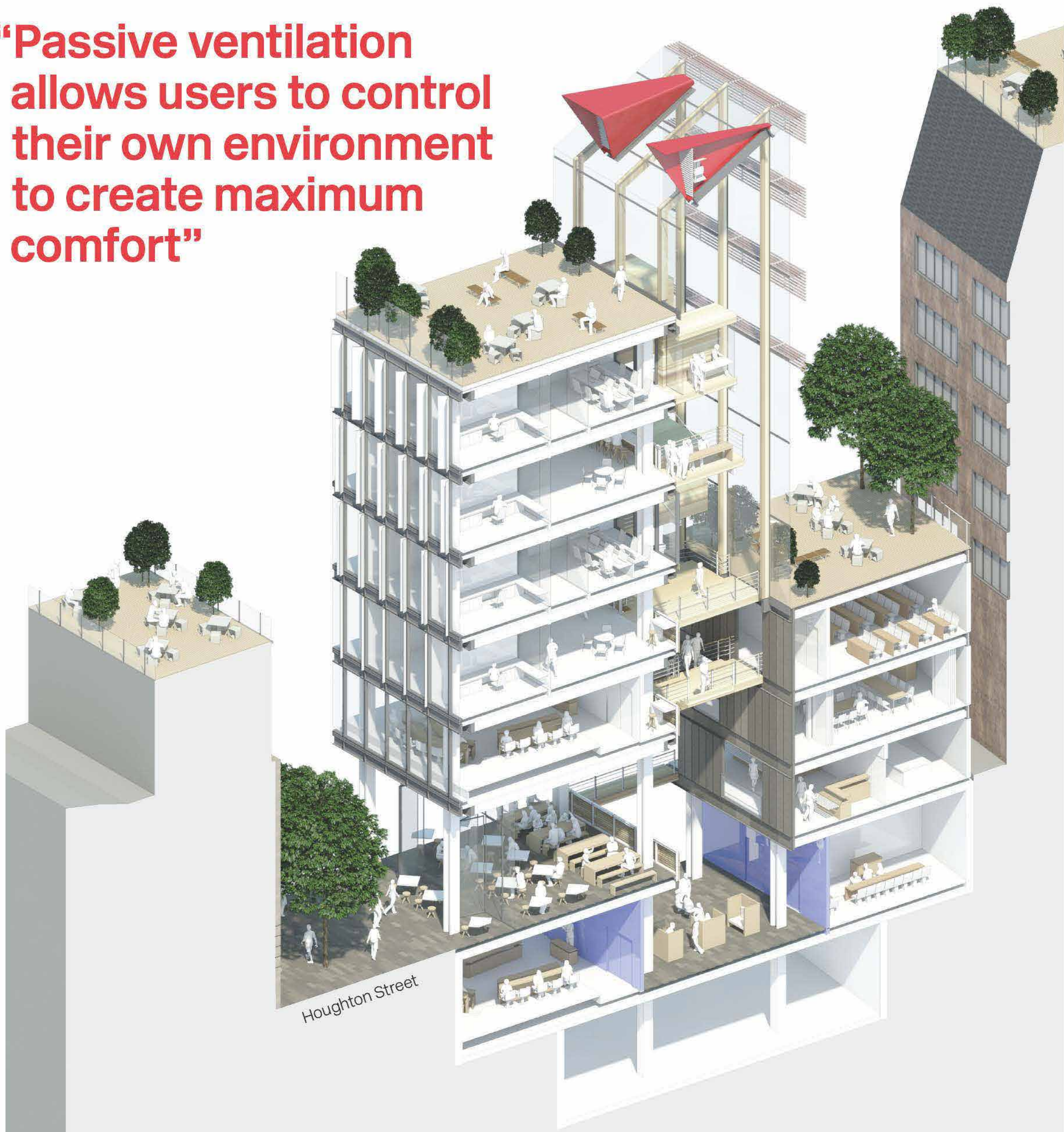
Cross section through the building
